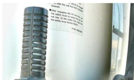
Figure 5: Latching hook lever safety pin location
