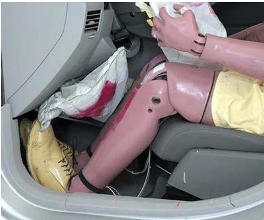
Figure A7: Example of a deployed knee airbag (photo from [airbagsystems.org](http://airbagsystems.org))
