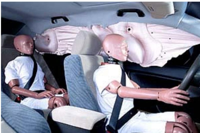
Figure A5: Curtain Airbags deploy from side roof sill (photo from <http://world.honda.com>)
