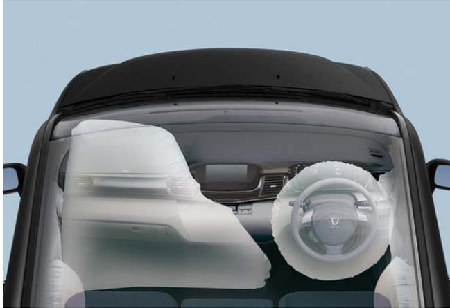
Figure A3: Frontal Airbags deploy from the steering wheel and dashboard (image from Honda.co.za)
