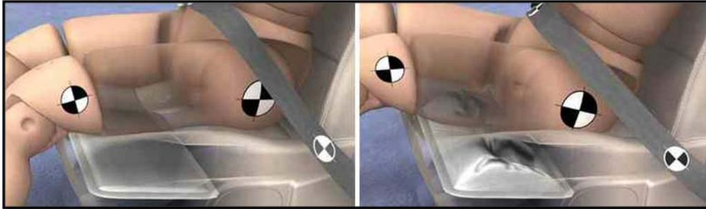
Figure A8: Anti-Submarining airbag un-deployed (left) and deployed (right) (image from [airbagsystems.org](http://airbagsystems.org)).
