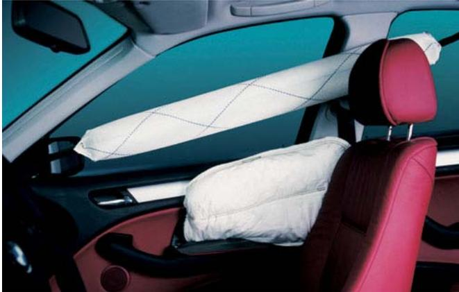
Figure A6: Tubular airbag used in conjunction with a thorax airbag (image from Mello, 2008)
