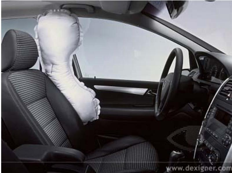
Figure A4: Deployed head/ thorax airbag (image from dexigner.com, 2005)
