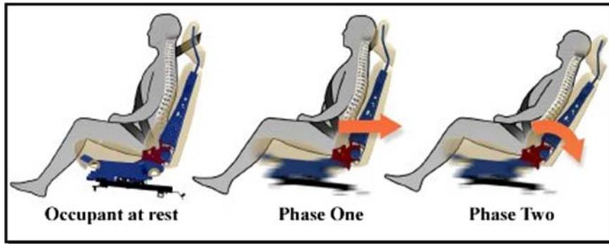
Figure A1: Phases of the WHIPS seat (Image from Clarke, 2008)
