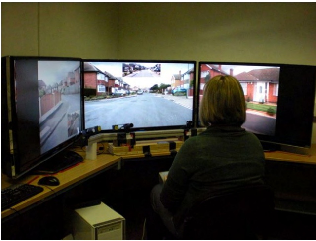
Fig. 1. Multi-screen set-up for the three-screen hazard perception test.
