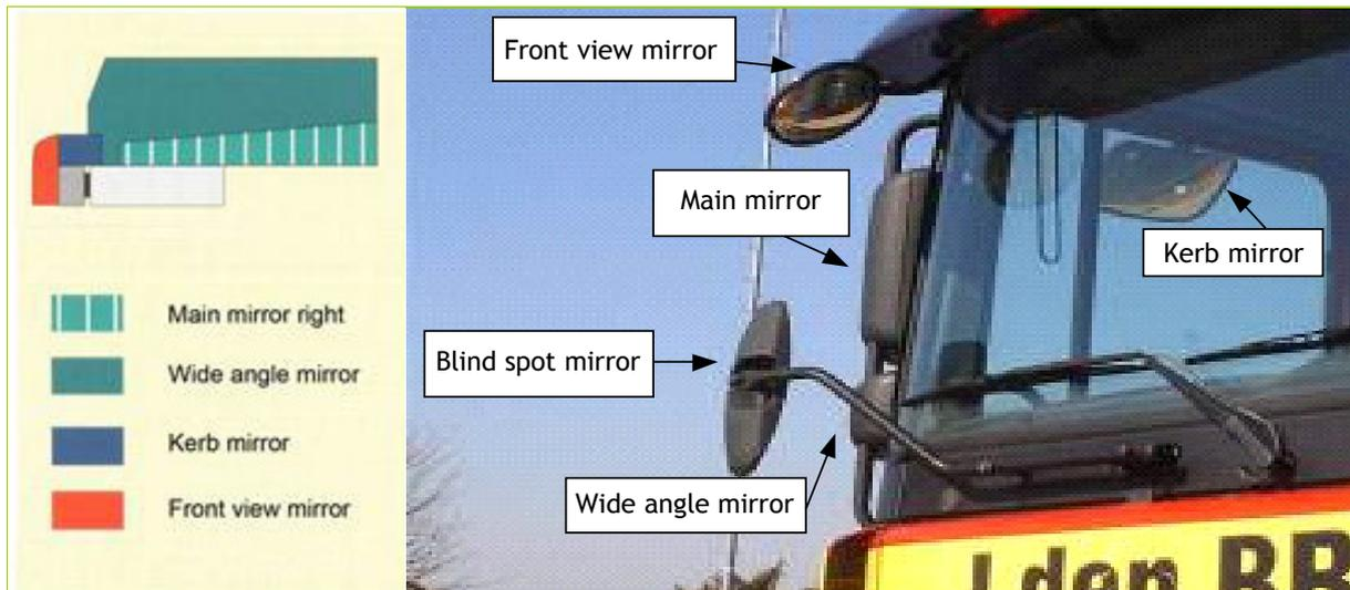
Figure 1. On the left a top view of the required field of vision for lorries according to the new EU requirements for new lorries from 2007 (Ministry of Transport, Public Works and Water Management, 2006). On the right a mirror configuration of a lorry before 2007 with a blind spot mirror (Schoon, Doumen & De Bruin, 2008).
